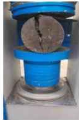
Figure 7: Split Tensile Strength Test.
